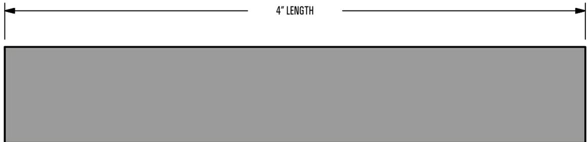
FABRICATE FROM SAME MATERIAL AS STANDING SEAM ROOF
